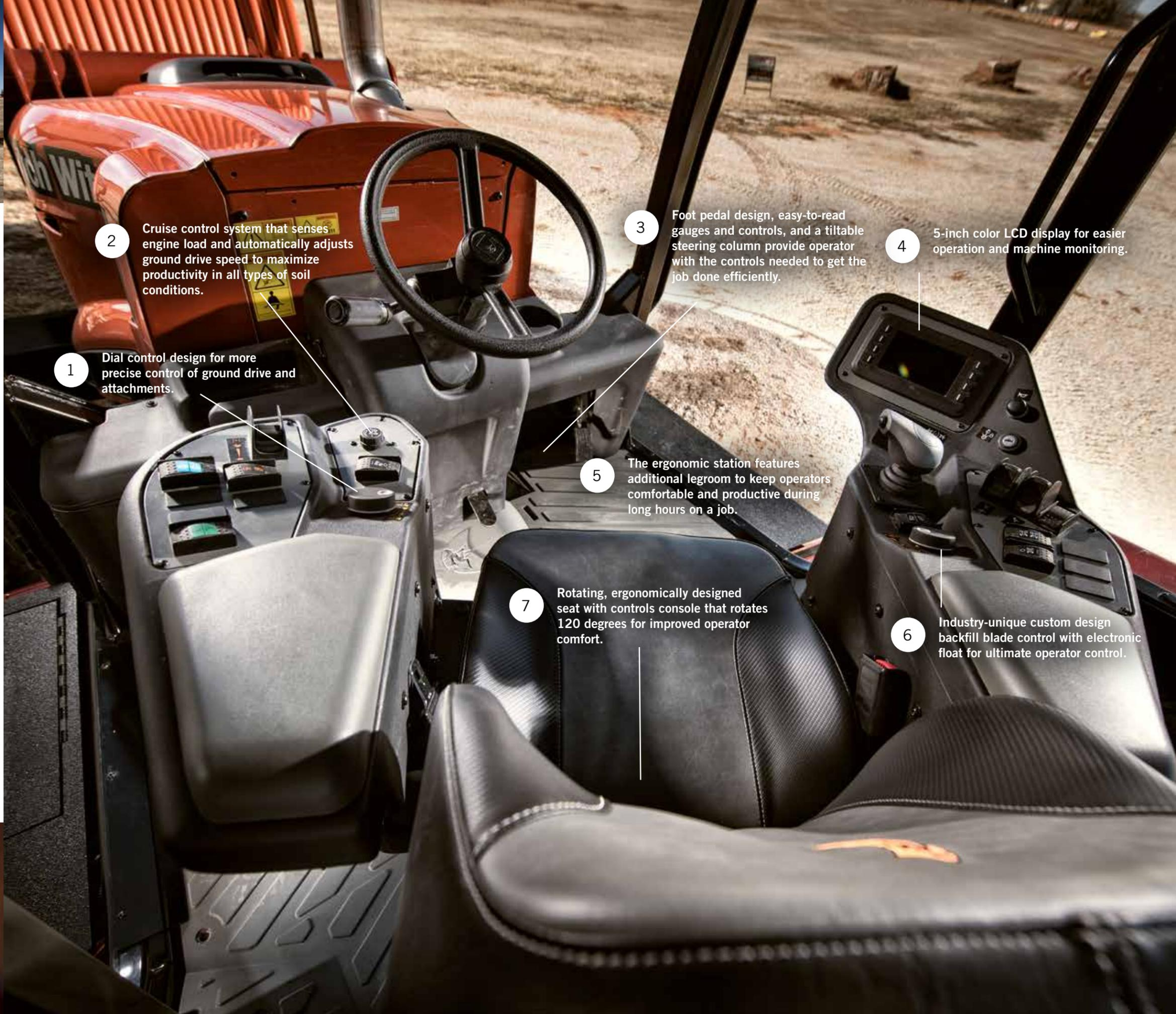
2 Cruise control system that senses engine load and automatically adjusts ground drive speed to maximize productivity in all types of soil conditions.
