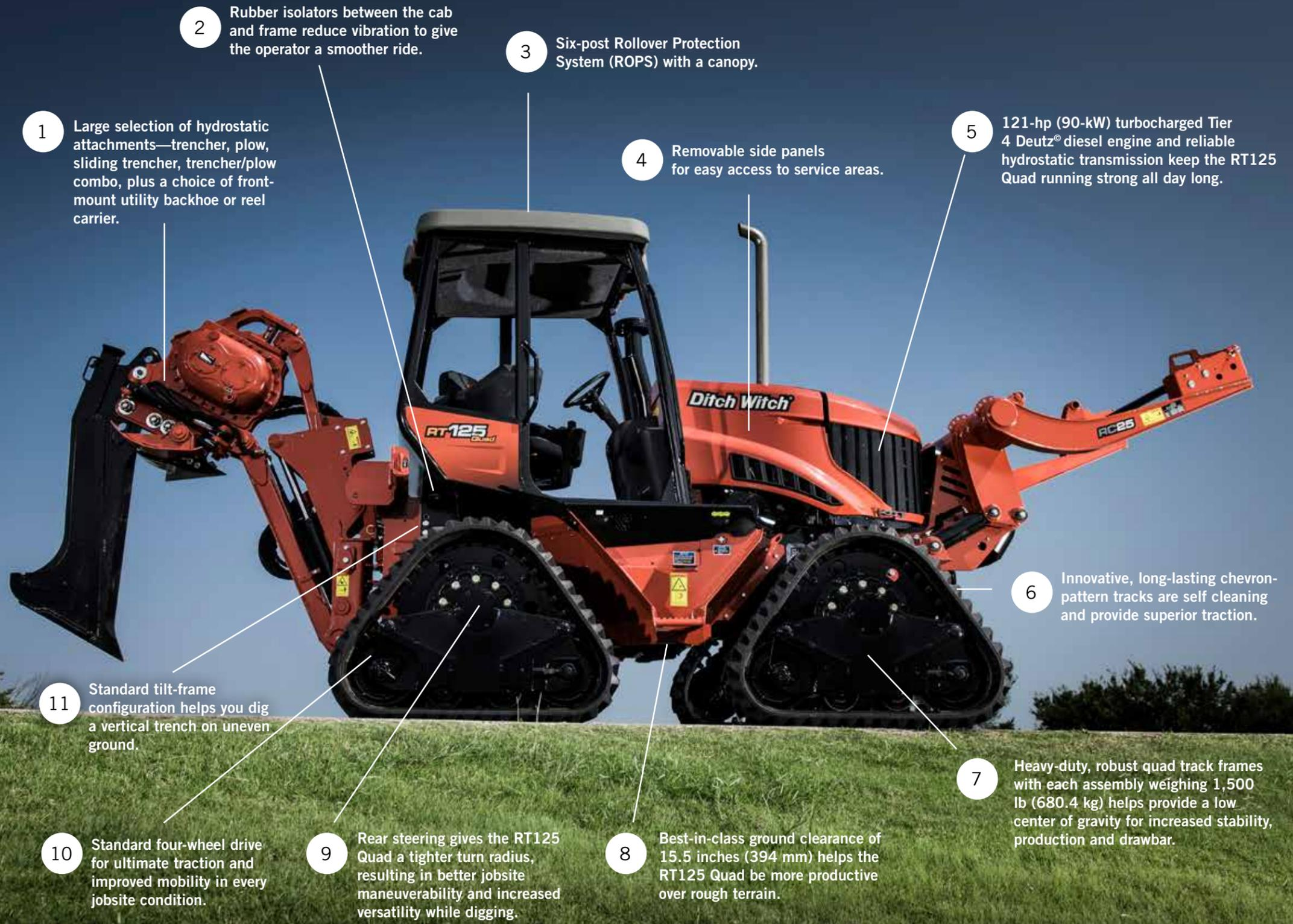
1 Large selection of hydrostatic attachments—trencher, plow, sliding trencher, trencher/plow combo, plus a choice of front-mount utility backhoe or reel carrier.
